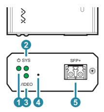
1 Power LED: This LED will illuminate to indicate the unit is on and receiving power.
